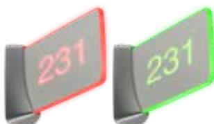
**Room Availability Indicators** placed outside meeting spaces, huddle rooms, offices, and other common spaces allow to confirm whether the space is free prior to entering. The act of physically walking into a room will switch the indicator sign to "occupied." These can be used as part of the Crestron scheduling system, or can be combined with the Crestron control platform to customize functionality.
